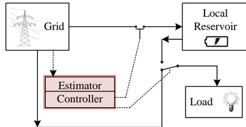
Fig. 1. Fundamental architecture of a peak shaving system.
