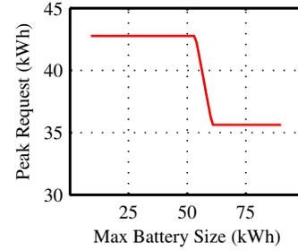
Fig. 5. Effect of battery size on the peak request
